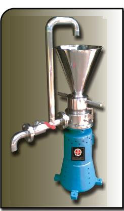
The material is fed through a SS Hopper and is forced between the Rotor and Stator where the material is sheared, dispersed, mixed and homogenized.
